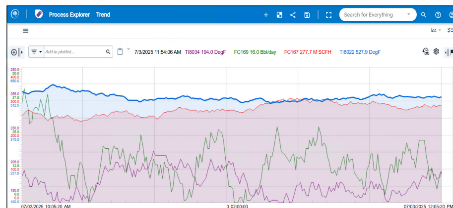
Figure 1: Time series trending of Aspen IP.21 data with many functions: zoom, annotations, comments, time shifting, control of pens and more.
